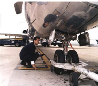
The pilot tests a number of safety systems, Taylor says. Instruments, gauges, and the actual aircraft are all closely inspected. "Pilots do a physical inspection of the airplane, inside and out," he says. "We look at the obvious things, like whether the engines are there, but we also look for more subtle factors such as tire pressure. In a car, a small variance in pressure isn't a big deal, but in a plane that weighs so much, a little change in pressure can be a major
